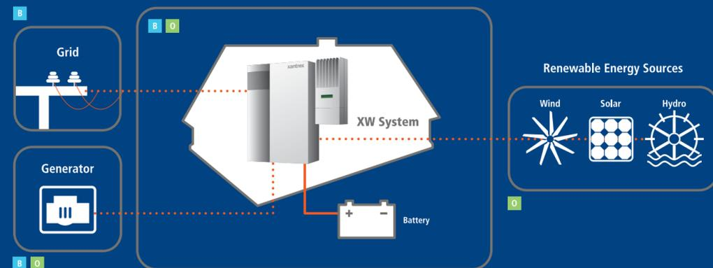
The XW Hybrid Inverter/Charger (XW) is a true sine wave inverter/charger that incorporates a DC to AC inverter, a battery charger, and an AC auto-transfer switch. It is the foundation for battery-based residential and commercial applications up to 18 kilowatts (kW). Designed for off-grid and back-up applications, the XW can operate with generators and renewable energy sources to provide full-time or backup power.
